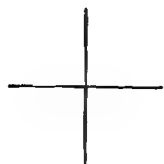
LINES ARE NOT CONNECTED
