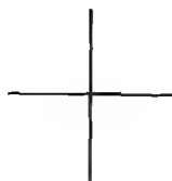
LINES ARE NOT CONNECTED
