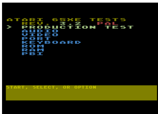
Figure 3-6. Main Menu display(on left 65XE NTSC, on right 130XE PAL)
